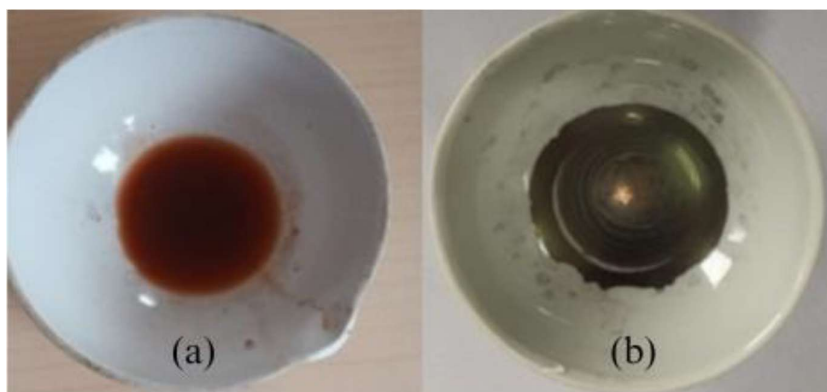
Figure 3. (a) Precipitate of silver nanoparticles (b) Dry silver nanoparticles
